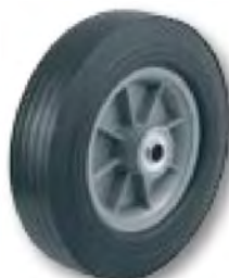
WH 64 10 X 2 1/2" S.R. 5/8" B.B. 3 1/4" Hub Width 400 lbs. Cap. Wt. 5 3/4 lbs.
