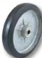
WH 77 8" X 1 5/8" M.O.R. 5/8" B.B. 2" Hub Width 450 lbs. Cap. Wt. 2 1/4 lbs.
