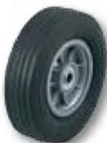
WH 14 8" X 2 1/4" S.R. 5/8" B.B. 2 1/4" Hub Width 400 lbs. Cap. Wt. 3 1/2 lbs.
