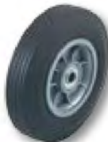
WH 85 8" X 2" S.R. 5/8" B.B. 2 1/4" Hub Width 300 lbs. Cap. Wt. 3 1/4 lbs.
