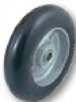
WH 56 8" X 2 1/4" Balloon Cushion 3/4" B.B. 2" Hub Width 450 lbs. Cap. Wt 4 lbs.
