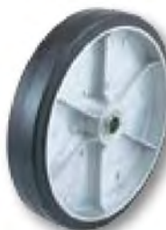
WH 62 10" X 2" M.O.R. 5/8" B.B. 2 1/4" Hub Width 600 lbs. Cap. Wt. 5 1/2 lbs.
