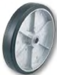
WH 68 10" X 2" M.O.R. 3/4" B.B. 2 1/4" Hub Width 600 lbs. Cap. Wt. 5 1/2 lbs.
