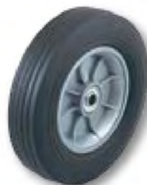
WH 60 10" X 2 1/2" S.R. 5/8" B.B. 2 1/4" Hub Width 400 lbs. Cap. Wt. 5 1/2 lbs.
