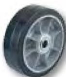
WH 63 6" X 2" M.O.R. 5/8" B.B. 2 1/4" Hub Width 460 lbs. Cap. Wt. 2 1/4 lbs.
