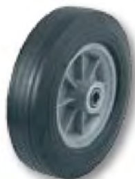
WH 83 10" X 2 1/2" S.R. 3/4" B.B. 3 1/4" Hub Width 400 lbs. Cap. Wt. 6 lbs.
