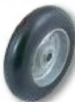
WH 55 8" X 2 1/4" Balloon Cushion 5/8" B.B. 2" Hub Width 450 lbs. Cap. Wt 4 lbs.
