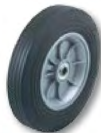
WH 86 10" X 2" S.R. 5/8" B.B. 2 1/4" Hub Width 300 lbs. Cap. Wt. 4 3/4 lbs.
