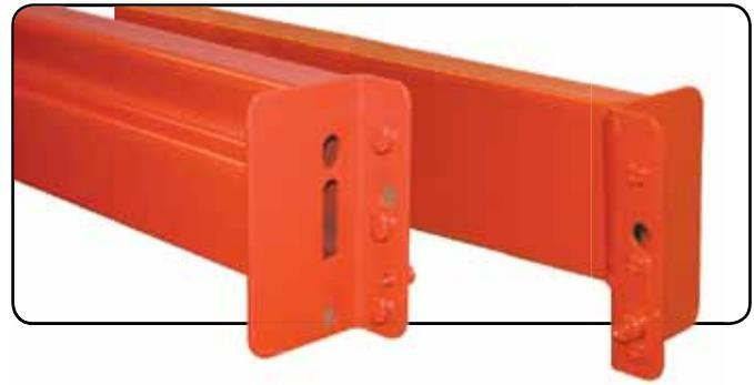
**Three-Point Safety Catch** – Each beam has 3 rugged studs (4 on heavy-duty) that engage the tapered keyhole slots in the
