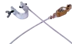
Part# 272031 All Purpose Bond Wire: For bonding drums to each other, to containers being filled, and to racks. Three-foot-long heavy duty wire rope with "C" clamp on one end and alligator clip on the other. Minimum order Qty. 5.
